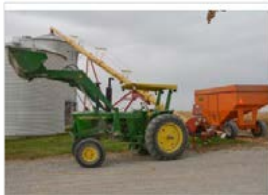
Tractors with rollover protection structures and shields/protective collars on power takeoff shafts help protect farmers during harvest. (DTN/Progressive Farmer photo by Matthew Wilde)
